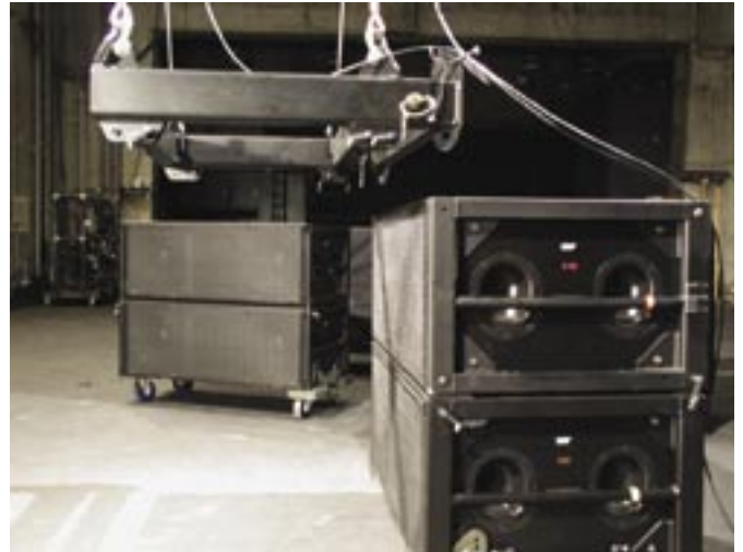
Figure 13. The MTG-3D Top Grid raised for pick up of the first M3D block
